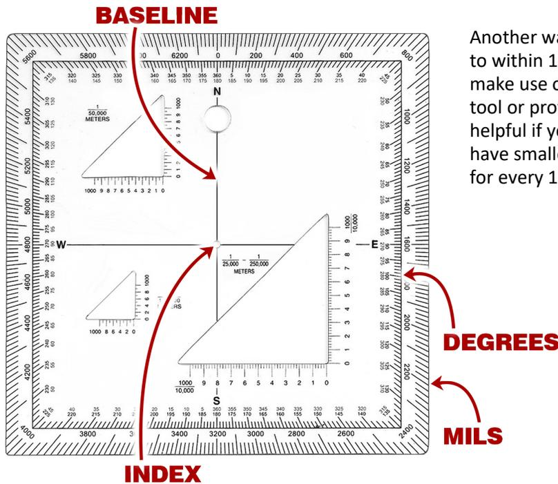
Another way to locate a point to within 100 meters is to make use of a coordinate scale tool or protractor. This is helpful if your map does not have smaller squares marked for every 100 meters.
